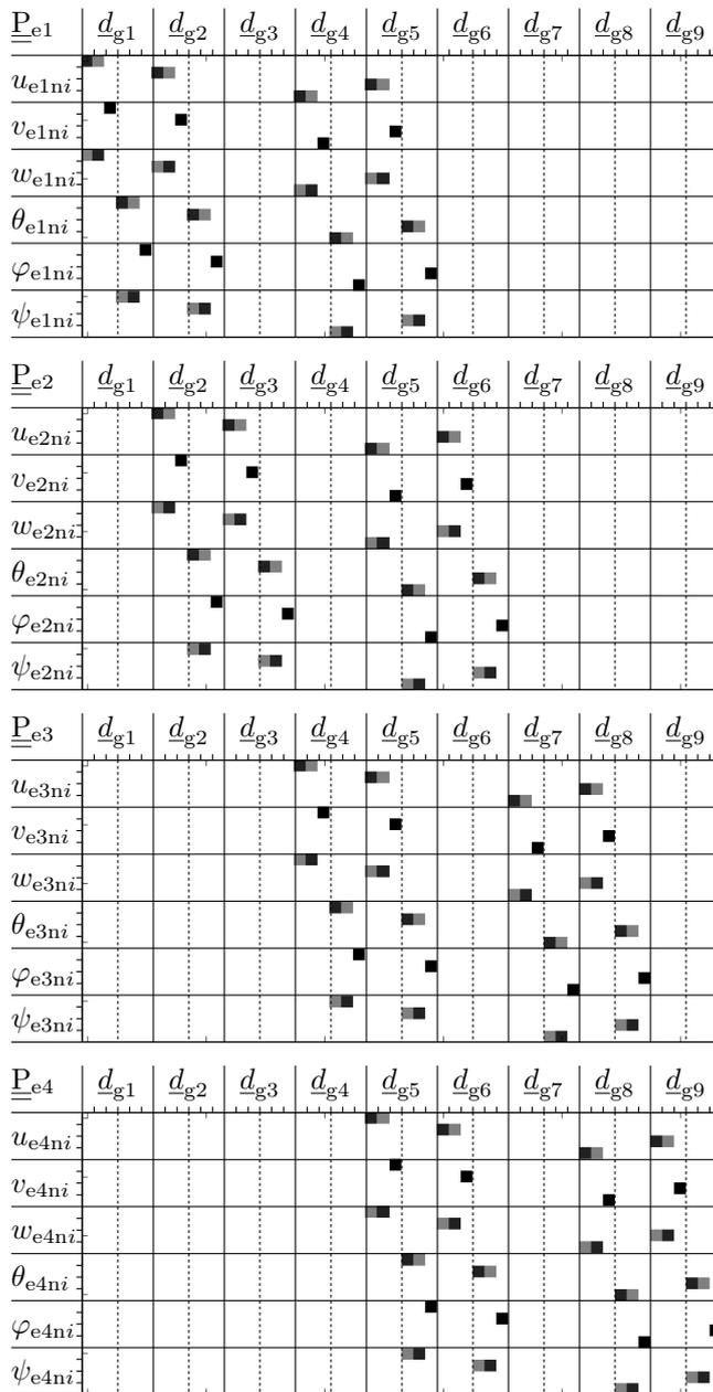
Figure 3: A grayscale representation of the terms of the four  $\underline{P}_{ej}$  mapping matrices associated the elements of Fig. 1. The colormap spans from white (zero) to black (one); the lighter and the darker grey colors represent terms that equate in modulus  $\sin 30^\circ$  and  $\cos 30^\circ$ , respectively.
