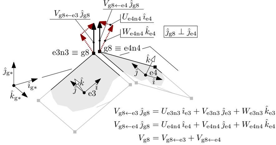
Figure 4: Accumulation of elemental nodal actions at global nodes.
