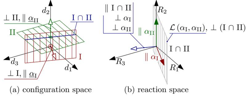
Figure 7: Allowed system configurations and constraint reactions for the pedagogical example of Fig. 6. The allowed displacement sets are easily derived as the homogenous counterpart of (a), and are not represented here.
