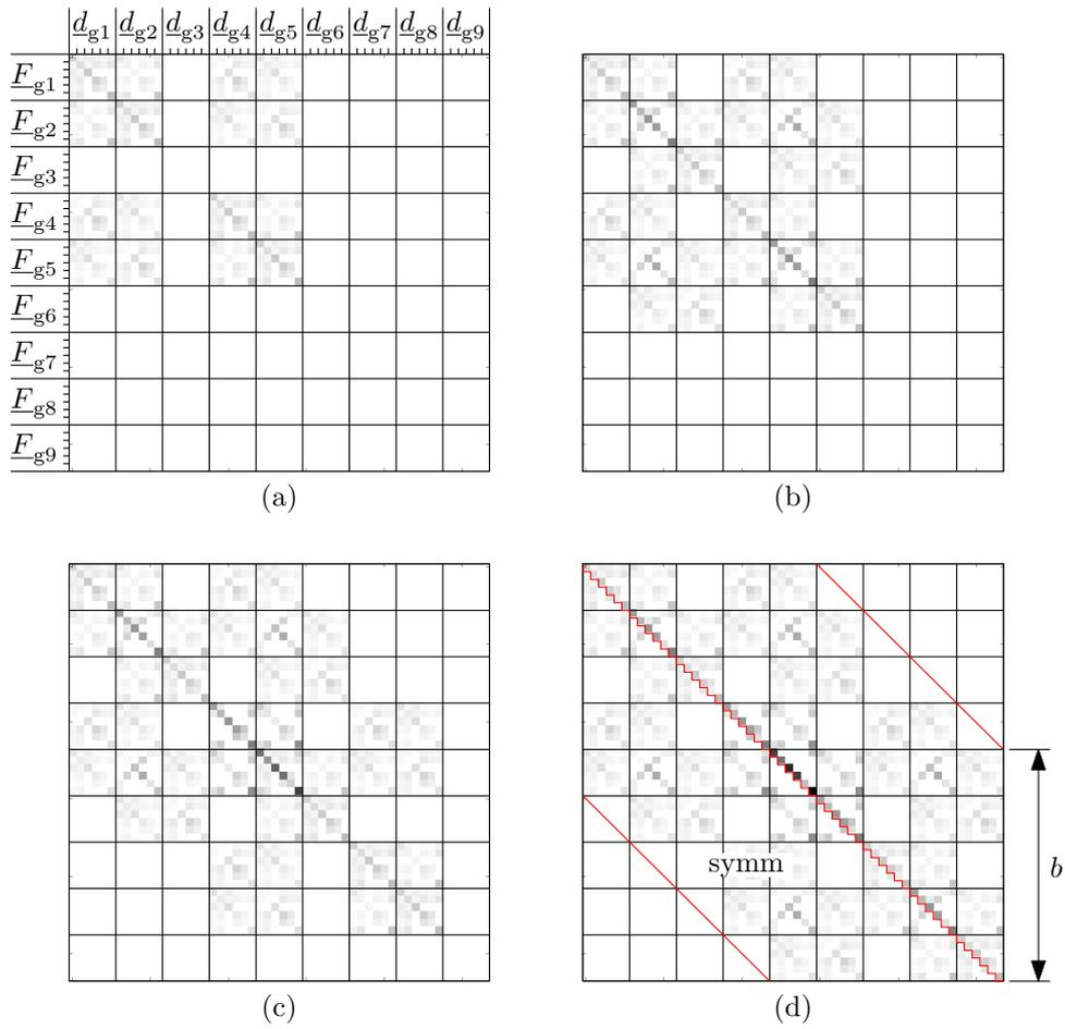
Figure 5: Graphical representation of the assembly steps for the stiffness matrix of the Fig. 1 structure. The zero-initialized form for the matrix that precedes the (a) step is omitted.
