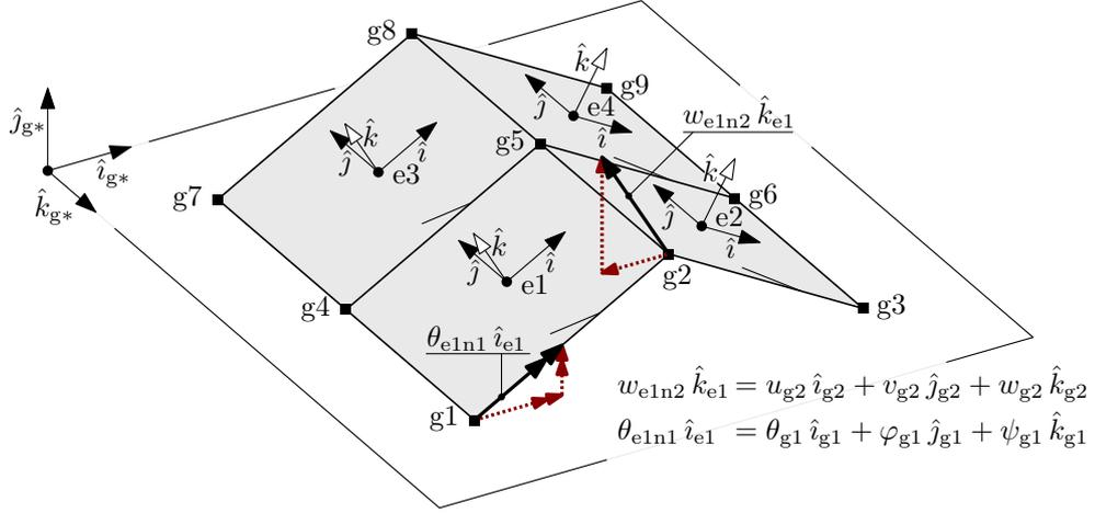
Figure 1: A simple four-element, roof-like structure employed in discussing the assembly procedures. The elements are square, thick plates whose angle with respect to the global  $XY$  plane is  $30^\circ$
