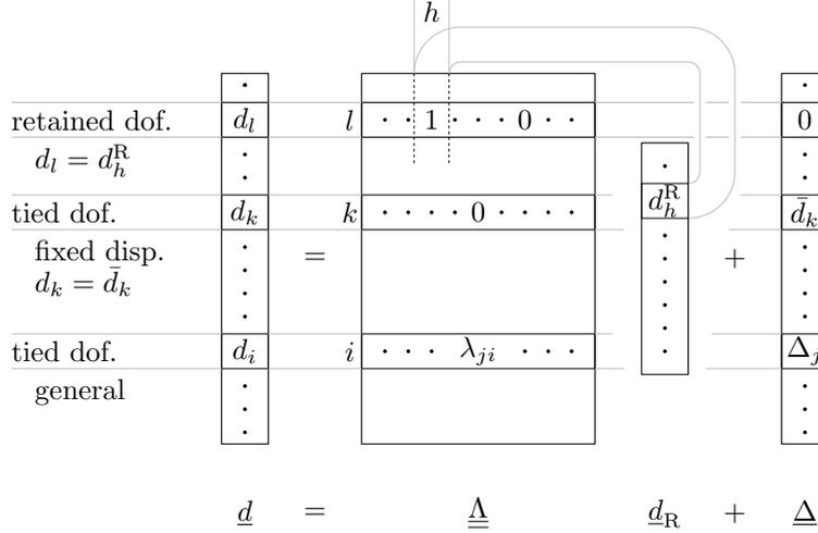
Figure 8: Graphical representation for the  $\underline{\Lambda}$  matrix in Eq. 20; representative matrix rows are illustrated for a retained DOF, and for two tied DOFs, namely a fixed displacement subcase, and the general case.
