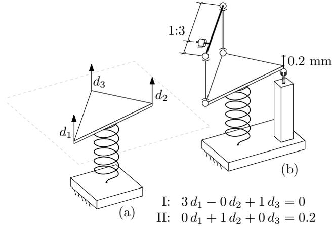
Figure 6: A pedagogical elastic three d.o.f. system, (a), subject to a few kinematic constraints (b).
