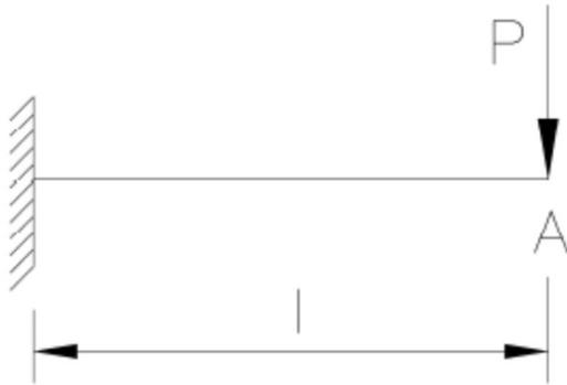
Considering a cantilever beam in steel loaded by a concentrated force  $P$  at the extremity called point A and fixed to the further extremity, evaluate the deflection of the beam at the point A ( $\delta_A$ ).
